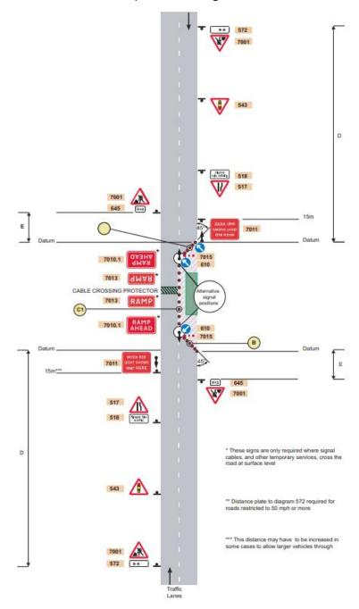
Diagram 1.1: Portable traffic signals on a two-lane single carriageway road
